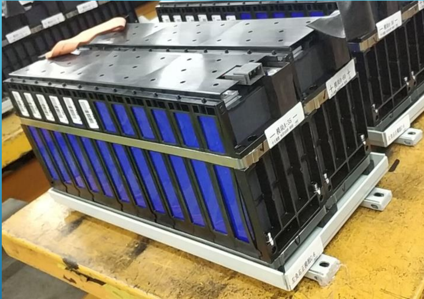
BATTERY PACKS MADE OF 3.2V 100AH CELLS
