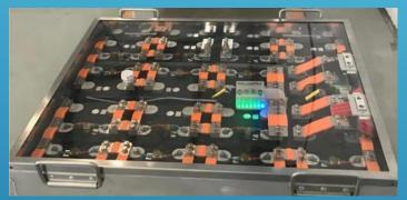
BATTERY PACKS MADE OF 3.2V 240AH CELLS
